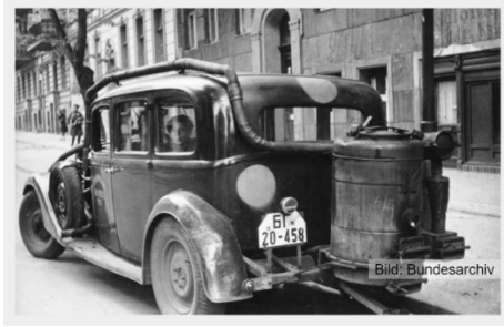
Abb. 9: Car at the 1950 th with wood gasification system.
