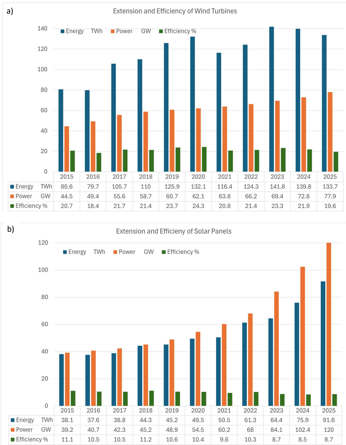
Fig. 4: Gross electricity generation (energy, Blue), installed nominal capacity (Orange) and efficiency (Green) a) of wind turbines, b) of photovoltaic plants in Germany.
